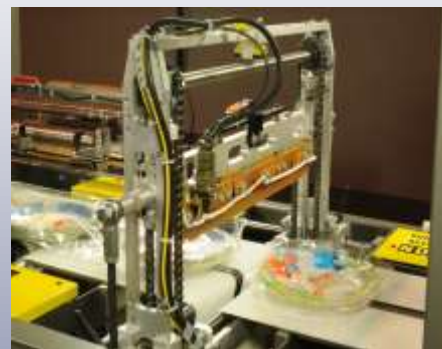
Multiple connecting points for seal frame and carriage provides support
